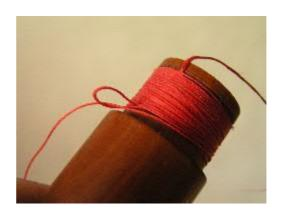
You can also secure the joint by using a needle to pass the end under the outer layers, in which case the initial loop is not necessary.
